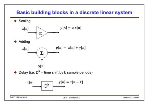
When building a linear discrete time system, we use only THREE operators:
