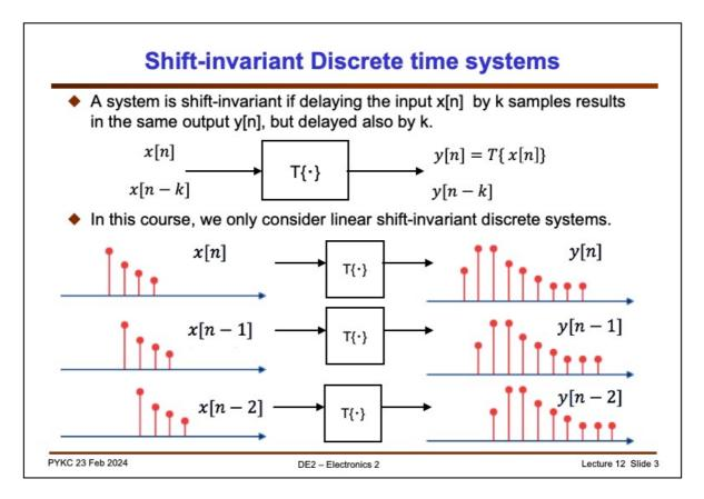
A shift-invariant system means that if you shift an input signal by k samples, the system response to x[n-k] is simply y[n-k]. It essentially means that the signal can start any time, the output remains the same but with the same delay as the input.
