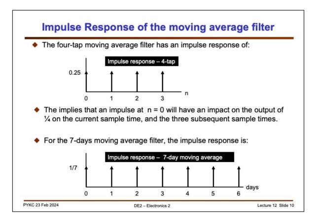
One important characterization of the 4-tap moving average filter is its impulse response. Plotted here is the output of the filter to an impulse at n=0. That is, if the input x[n] is an impulse a n=0, then its effect on the output y[n] is going to last of four sample periods at n=0, 1, 2, and 3. Since it is averaging, the weighting is 0.25 everywhere.
