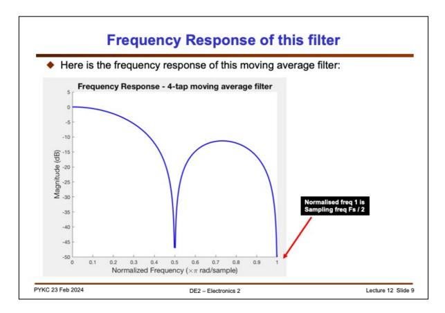
We can computer the frequency response of this simple 4-tap FIR or moving average filter with the following transfer function:
