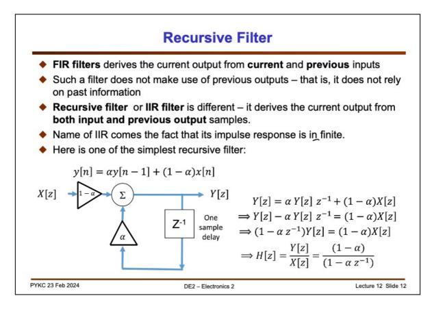
Let us now consider a completely new class of filter. Here we have a filter that derives the output from both inputs and past output samples. The simplest form is the one shown here – known as a first-order **recursive** filter.
