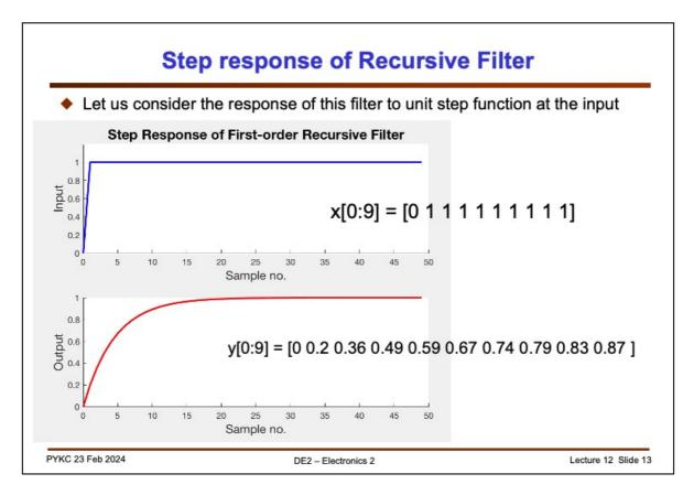
Now let us consider what output we get if we apply a unit step function at the input. The output is known as the step response of this filter.
