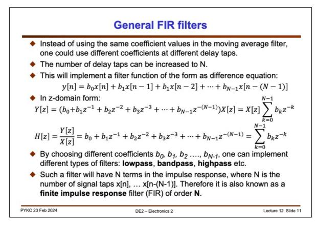
The moving average filter we used previously only considered 4 input sample values (we call this a "4-tap" filter, tapping into only 4 signal values). Instead of 4-tap, one can choose to perform the moving average over K-taps.
