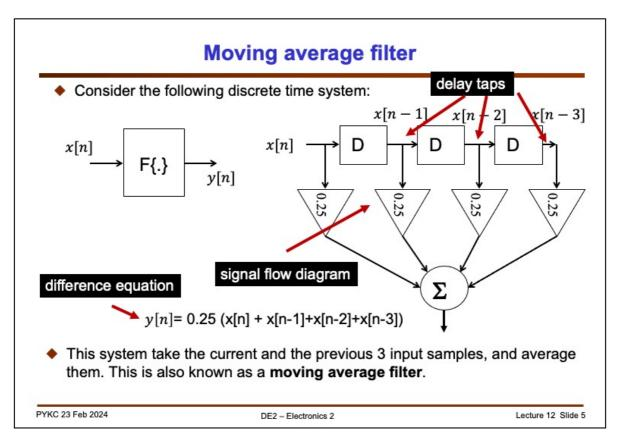
Consider a simple discrete time system which takes the current and three previous input samples, and calculate the average value:
