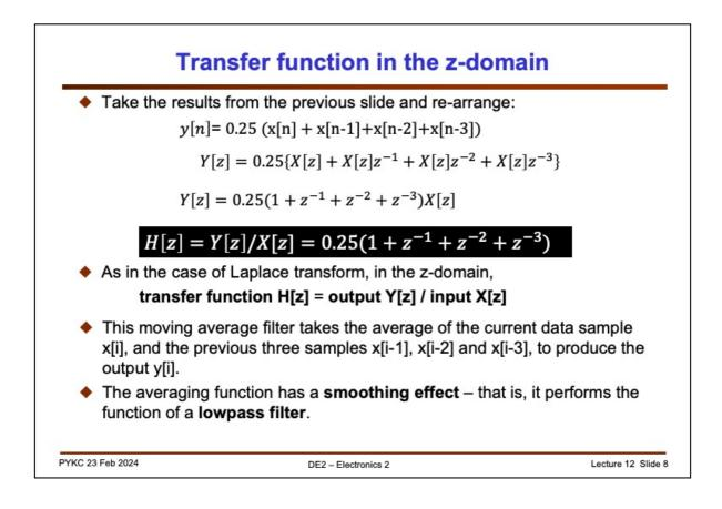
From the previous slide, we can compute Y[z]/X[z], and obtain the transfer function H[z]:
