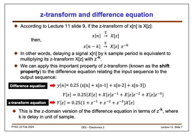
The third method of representing a discrete time system is to use z-transform to represent the delay operators. Again, I will discuss the mathematical basis of z-transform in a later lecture. For now all you need to know (and trust) is that delay a signal x[n] by k sampling periods to give x[n-k] is the same as multiplying the z-transform of the signal X[z] by the factor  $z^{-k}$ .
