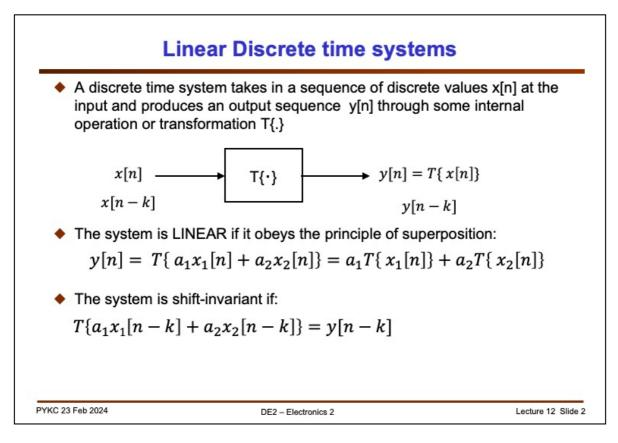
Let us first consider a linear discrete time system shown here as  $T{.}$ . ({.} is to indicate that T is an arbitrary system.). The system takes in the input sequence x[n] and produces the output sequence y[n].
